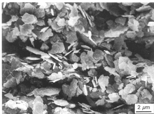
Figure 3 Scanning electron micrograph of the product obtained by the oxidation of iron powders in 0.2 M \text{Ba}(\text{OH})_2 –5 M NaOH mixed solution at 300 °C and 3 MPa oxygen for 2 h.
